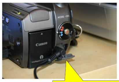
You'll open a small plastic protector under the mode dial to plug the camera into the power adapter.
