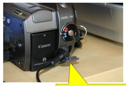
You'll open a small plastic protector under the mode dial to plug the camera into the power adapter.
